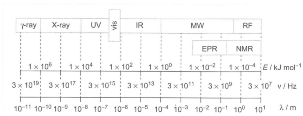
**Fig. 2.1** ESR spectroscopy and the electromagnetic spectrum. The subdivision of the spectrum is based on the wavelength and the corresponding frequency and energy. ESR spectroscopy operates with smaller wavelengths than NMR spectroscopy<sup>1</sup>.
