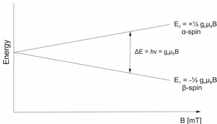
**Fig. 2.5** Lifting of the degeneracy by increasing the magnetic field strength results in electron Zeeman splitting and two electron Zeeman levels separated by  $\Delta E$ , denoted as  $E_1$  and  $E_2$ . A spin transition from the lower energy level to the higher energy level is induced when an electromagnetic radiation with a matching frequency is irradiated to fulfill the resonance condition.
