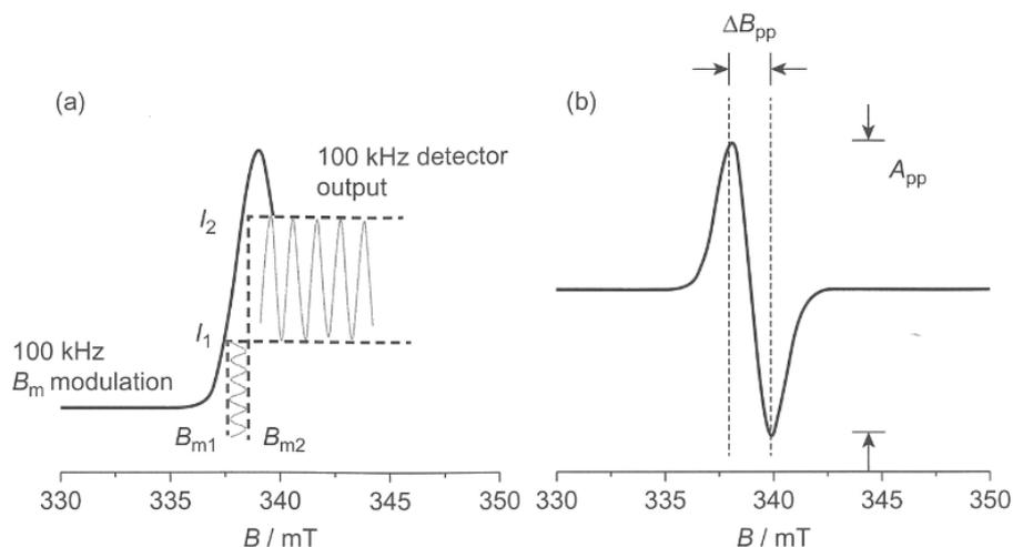
**Fig. 4.2** Absorption spectrum (in a) and first derivative profile (in b) as a result of field modulation. The detector output oscillates with the frequency of the field modulation. The peak-to-peak linewidth  $\Delta B_{PP}$  is the field difference between the points of inflection in the absorption spectrum<sup>2</sup>.
