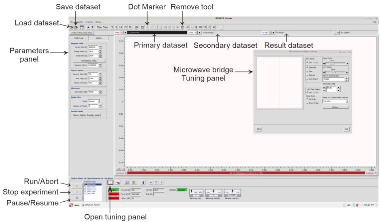
**Fig 6.1** The Xenon software for controlling the EMXnano spectrometer.
