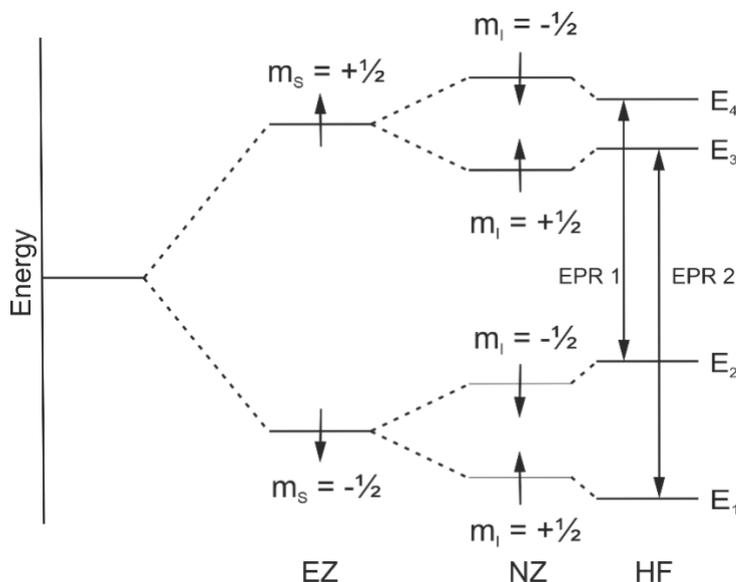
**Fig. 2.6** Energy level diagram resulting from electron Zeeman interaction (abbreviated with EZ), nuclear Zeeman interaction (NZ), and hyperfine interaction (HF) for a  $S = I = 1/2$  system. The CW EPR spectrum shows two transitions, which are labeled as EPR1 and EPR2.
