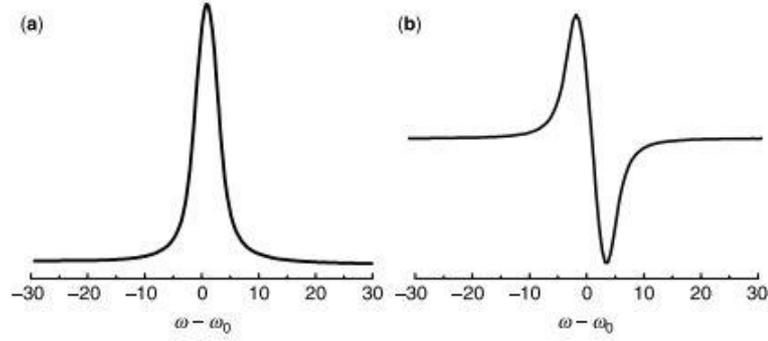
**Fig. 2.2** An example of an ESR spectrum, represented as an absorption curve in (a) and as the first derivative in (b). The expression  $\omega - \omega_0$  represents the deviation of the microwave frequency from the resonance frequency<sup>1</sup>.
