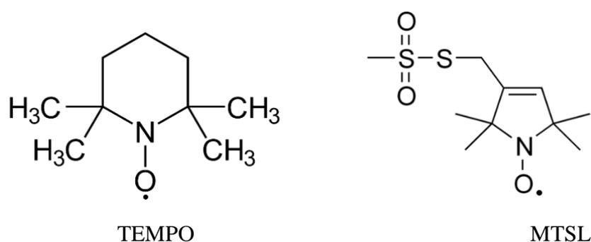
**Fig. 1.1** Chemical structure of the nitroxide spin labels used for the experiments. (Left) TEMPO (2,2,6,6-tetramethylpiperidine 1-oxyl). (Right) MTSL (1-oxyl-2,2,5,5-tetramethyl- $\Delta^3$ -pyrroline-3-methylmethanesulfonate).
