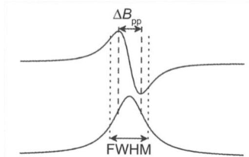
**Fig. 2.8** Linewidth of a CW ESR spectrum shown as the full width of half maximum (FWHM) for the absorption spectrum and as the peak-to-peak linewidth  $\Delta B_{pp}$  for the spectrum in first derivative mode<sup>1</sup>.
