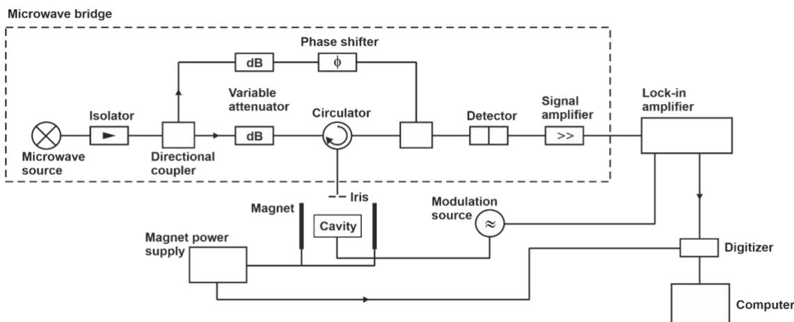
**Fig. 4.1** Simplified construction representing a typical CW ESR spectrometer. The sample to be measured is placed in the resonator or cavity (Adapted from 1).
