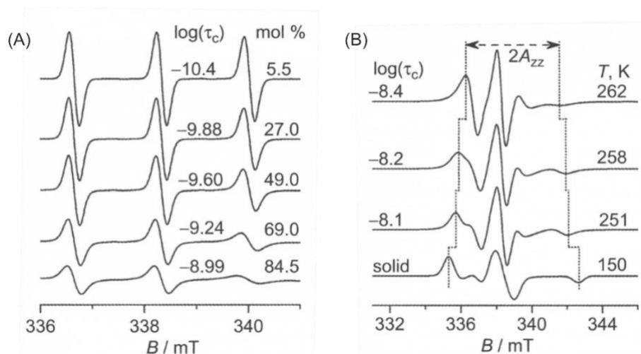
**Fig. 2.9** Effect of (A) viscosity and (B) temperature on the line width of the ESR spectra.
