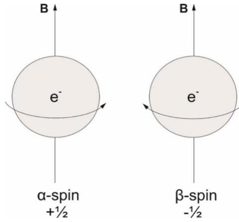
**Fig 2.4** The two oppositely oriented electron magnetic dipole moments with respect to the magnetic field, which arise due to the two allowed values for  $m_S$  corresponding to the  $\alpha$ -spin state (left) or the  $\beta$ -spin state (right).
