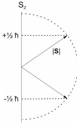
**Fig. 2.3** Vector representation for the quantized spin angular momentum  $\mathbf{S}$ .  $S_z$  represents the space quantization axis and coincides with the direction of the applied magnetic field.
