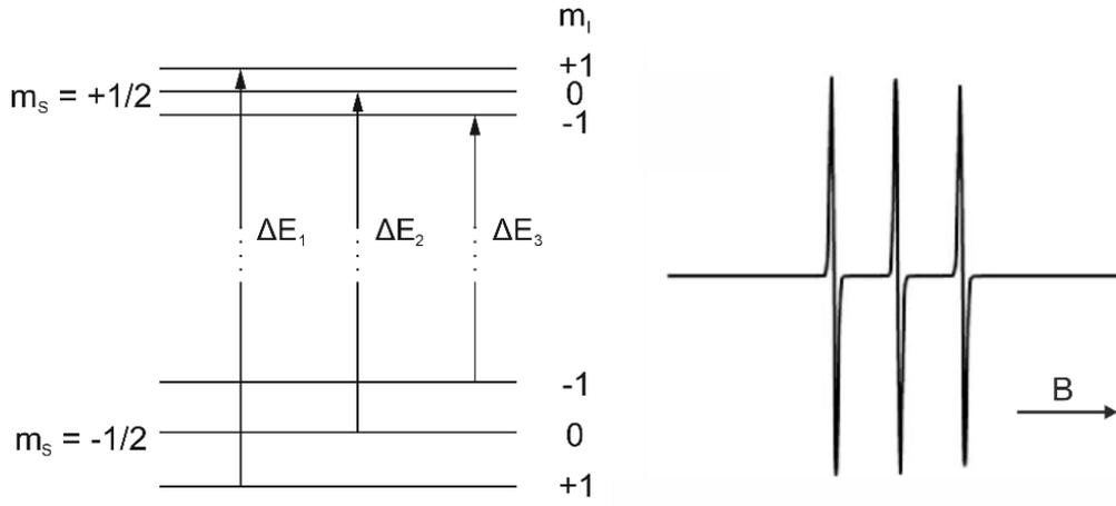
**Fig. 2.7.** Energy diagram (left) and resulting CW ESR spectrum (right) for a nitroxide radical with  $S = 1/2$  and  $I = 1$ . In the high field approximation, the three lines show roughly the same intensities because the energy difference between the ESR transitions (e.g.  $\Delta E_1 - \Delta E_2$ ) is small compared to the energy difference between the electron Zeeman levels denoted as  $m_s = +1/2$  and  $m_s = -1/2$ .
